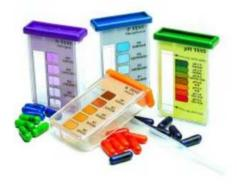
Figure 2 Soil pH – Nitrogen – Phosphorus – Potassium test kit
