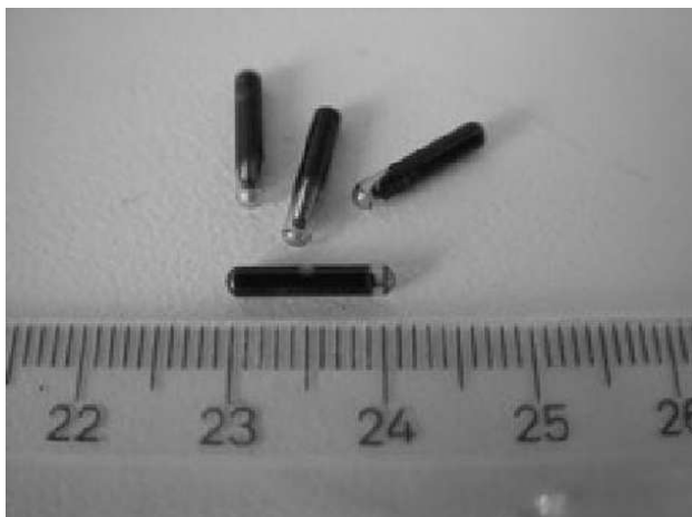
Figure 13 Image of RFID microchips
